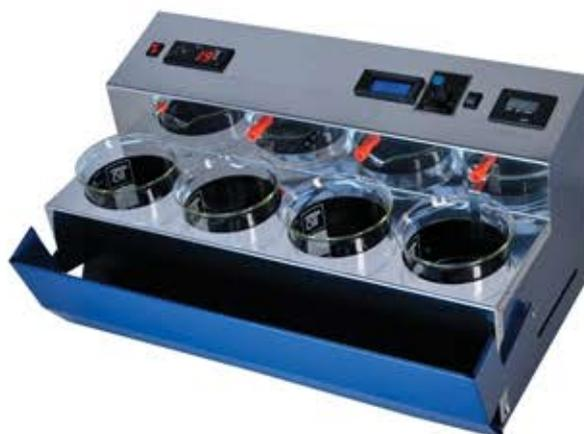
MACCHINA GALVANO PER LA GALVANOSTEGIA DI METALLI . CON QUESTA MACCHINA SI POSSONO EFFETTUARE BAGNI A ELETTROLISI A TAMPONE(PENNA) O IMMERSIONE PER DEPOSITI FLASH O A SPESSORE DI PICCOLI OGGETTI . MACCHINA ADATTA A GALVANIZZARE PICCOLI OGGETTI COME ANELLI, BRACCIALI , PENDENTI , ORECCHINI , SCHELETRATI E CAPSULE E PIUÙ IN GENERALE OGGETTI DI PICCOLE DIMENSIONI .
