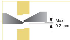
**Flush EDGE cut:** Expert shear cutting technology and a controlled edge misalignment of less than 0.2 mm to deliver a clean, smooth cut, on even the thinnest wires.
